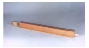
Students used organ pipes for a variety of acoustical exercises in the laboratory, including threshold determinations and research on the quality of tone. In the nineteenth century, Rudolph Koenig made the largest selection of organ pipes for research and demonstration.
