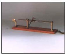
Experimenters used the Ergograph for a range of investigations. First they measured the physiological measures of muscular contraction, fatigue, endurance, strength and physical capacity or endurance. These tests were carried out under varying conditions, e.g. with stimulants, narcotics, poisons, exercise and special diets. In addition, experimenters measured the effects of mental tasks on physical endurance.
