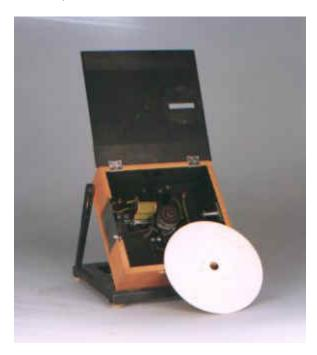
The Ranschburg Memory Device presents a series of visual stimuli successively, at a specified rate, to be memorized. Symbols, letters, numbers are written on the white disk, and temporarily revealed through the exposure slot. The Disk is driven in discreet steps by an internal motor.
